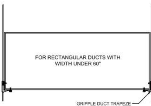
FOR RECTANGULAR DUCTS WITH WIDTH UNDER 60" RECTANGULAR DUCT INSTALLATION WITH GRIPPLE DT2
